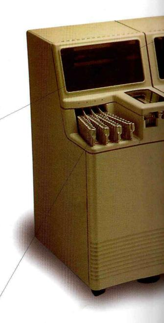
Sample Loading: Samples are placed in one of the four universal sample trays (any size primary collection tube or sample cup)
